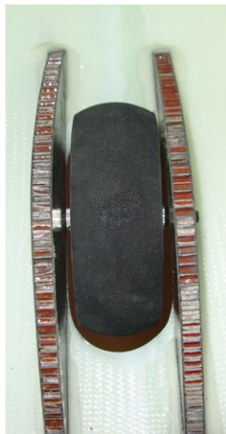
In Honeycomb-Platten gelagertes Bugrad
