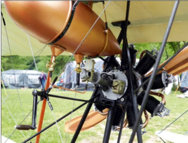
Tank, Motor, Anlasserkurbel: An den Modellen gibt's ganz schön was zu gucken
