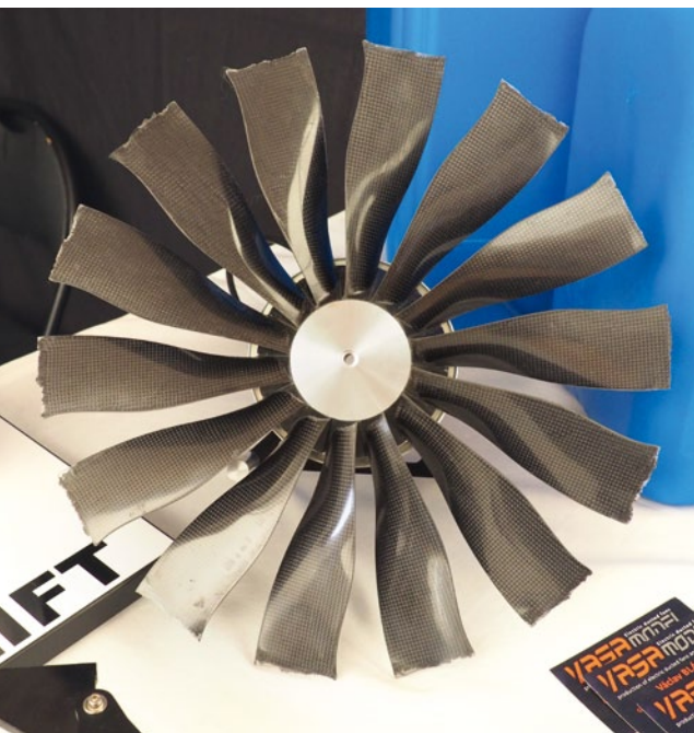
Rotor zu Vasas 300-Millimeter-Impeller
