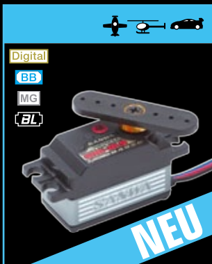
SRG-BLS Low Profile Brushless Servo für 1/10 Tourenwagen 0.05s/40° 6.0V | 7.6kg/cm 6V 40,5 x 21 x 26,5mm | 47g
