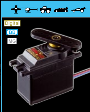
SRG-CZ Servo Super Response Coreless Torque-Servo 0.08s/40° 6.0V | 14.8kg/cm 6.0V 40.5x21x38mm | 63g
