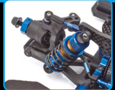
Updated suspension geometry with new composite material and optimized suspension arm length
