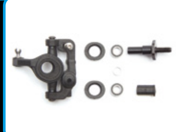
Steering and caster block insert system allows for easy caster and trailing axle adjustments
