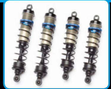
7075-T6 aluminum 16mm "Big Bore" threaded shocks with TiN coated 3.5mm shafts and larger diameter precision springs
