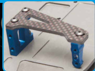
New floating servo mount improves symmetrical chassis flex
