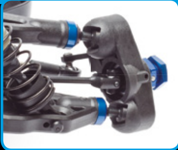
Front suspension features pillow ball uprights for increased adjustability and improved durability
