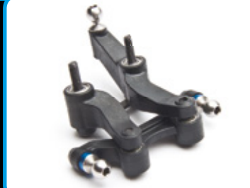
Updated steering system with horizontal ball studs for finer Ackermann adjustments
