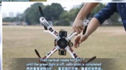
Then vertical rotate for 360° until the green light is off, calibration is completed. 然后垂直旋转360°, 直至绿灯灭掉, 垂直校准完成。
