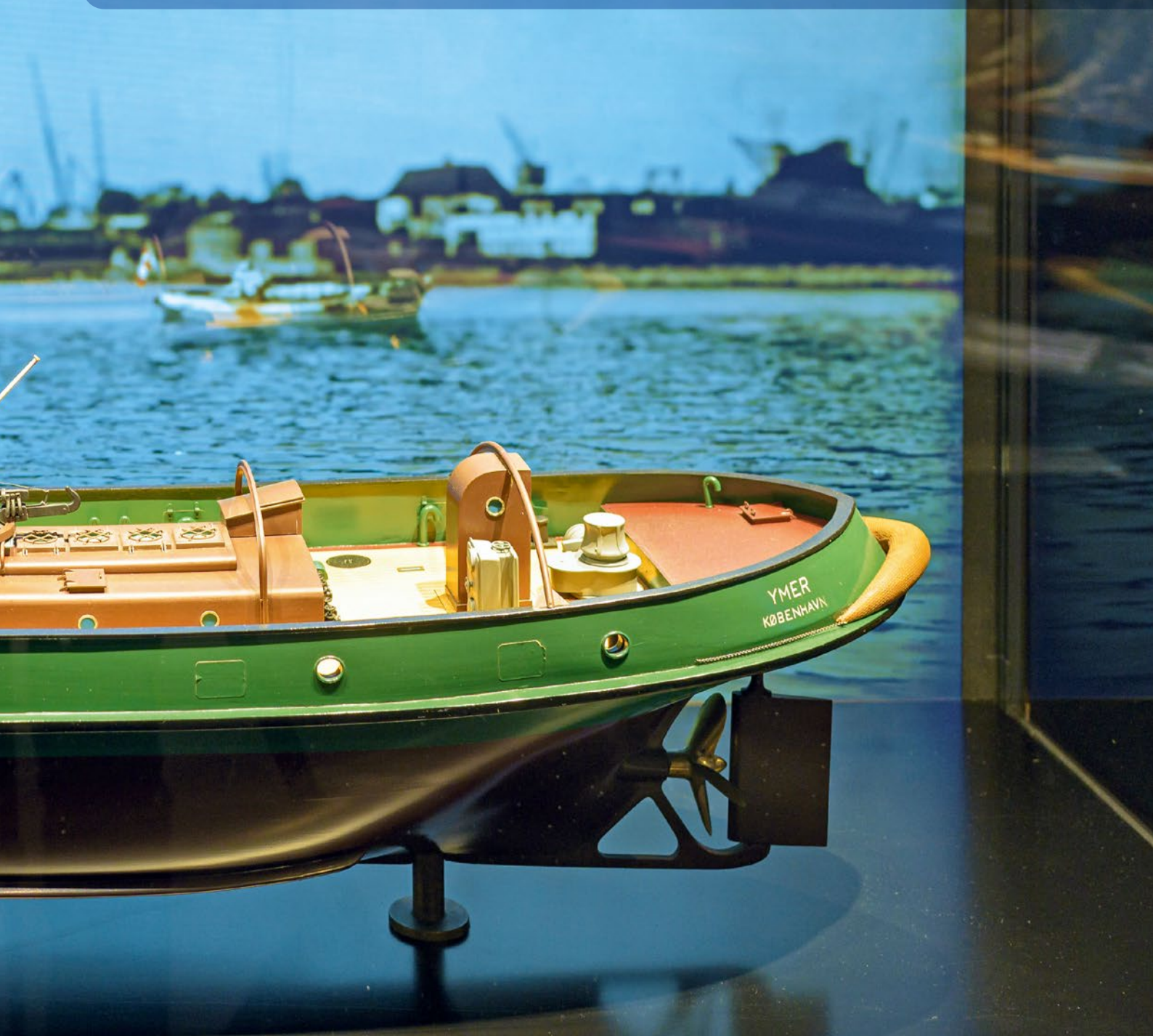
YMER The YMER is a tugboat – a ship that tows or pushes other ships. When the ship was built in 1942, the waters, ports and harbours of Denmark were still made of wood. The YMER, which was also built to break ice in the Copenhagen harbour, was made of steel. The YMER was not just any tugboat. It was the first fully welded ship in Denmark. The hull was welded together – whereas the hulls of other ships were assembled from planks. All-welded hulls are cheaper, lighter and more watertight. On the other hand, the steel needs to be of better and more uniform quality. As an extra fitness, the YMER was equipped with a telescopic funnel so that the tugboat could sail under the Knippelsbro bridge without any problems. Vessel: Tugboat | 91 GRT | built at the Aalborg Shipyard, 1942 | Det Forenede Bogserselskab
